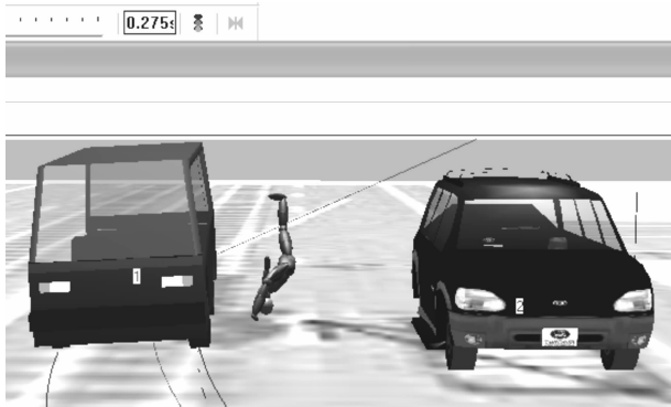
图 8 仿真 0.275 s 时刻人车相对位置 Fig. 8 The relative position of vehicle and pedestrian when t=0.275 s in simulation
